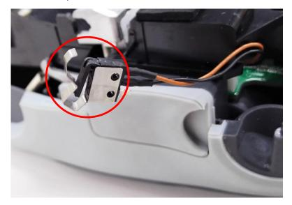
6. Place the open sensor on the side of media cover switch.
