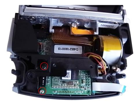
3. Disconnect the connector on the board.
