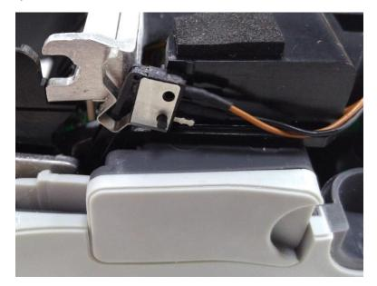
7. Lock the screw on the side of media cover switch.
