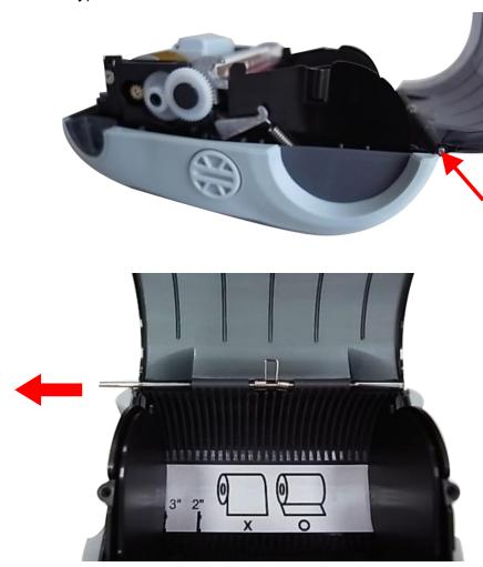
3. Use a tool to remove the shaft. Remove/Replace the media cover. (including the platen roller ass'y)
