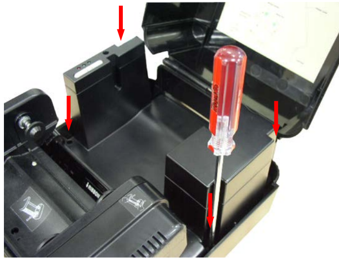
Remove screws of the label roll mount
