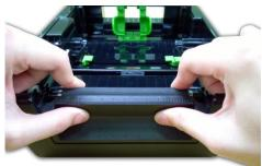
6. Hold the grounding cable onto the right side of the peel-off bar. Then, install the peel-off bar into both slots on front inner lower cover. Please install left side (with spring) first. Make sure the flat side of grounding wire is on right side as shown below.
