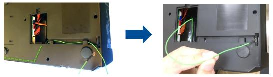
**5.** Open the printer top cover then open the print head mechanism. Remove the lower front panel.
