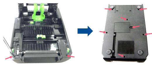
2. After removing the lower cover, remove two screws securing the main board on the lower inner cover. (no need to disconnect all the cables on the main board)
