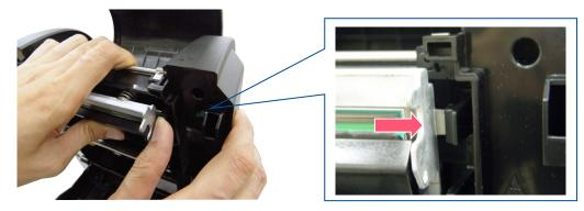
4. Disconnect printhead harness and ground cable to replace the printhead module.
