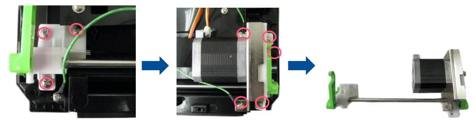
**5.** Remove one e-ring to replace stepping motor module.
