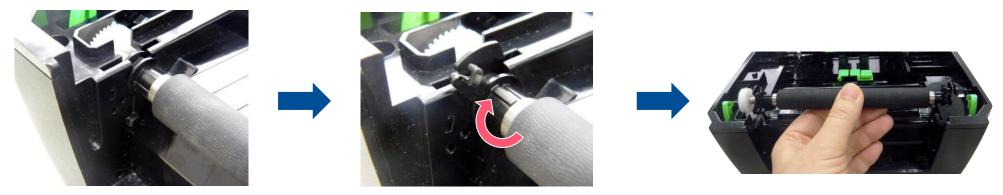
**3.** Take out the platen roller assembly to replace. Reassemble the parts in the reverse procedure.
