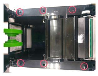
2. Remove the 10 screws on the ribbon base module.
