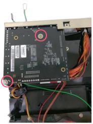
3. Disconnect the grounding connector next to the DC jack. Plug the peel-off bar grounding cable pin into the same connector.
