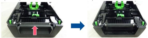
2. Disengage the platen holder tabs by pulling out the right side and left side tabs. Rotate the tabs into the forward position. (see picture below)
