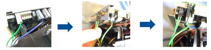
4. Install the lower cover by eight screws then pull the grounding cable through the opening. Put the grounding cable through the slot of the lower cover.
